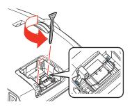
7. Lift up the lamp handle and gently pull the lamp out of the projector.
